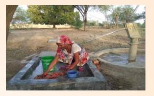
With the active participation of Pani Panchayat committee project has constructed 5 concrete washing platforms with Soak pit to mitigate water logging problem. It not only recharges the ground water with the waste water but also helps in maintaining cleanliness around the hand pump by providing a proper drainage system. Total 51 families are now able to access safe drinking water in hygienic condition due to these hand pumps linked to soak pits.
